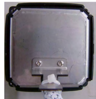
3) Close rear cover. Fasten cable to clamp with cable tie (supplied).
