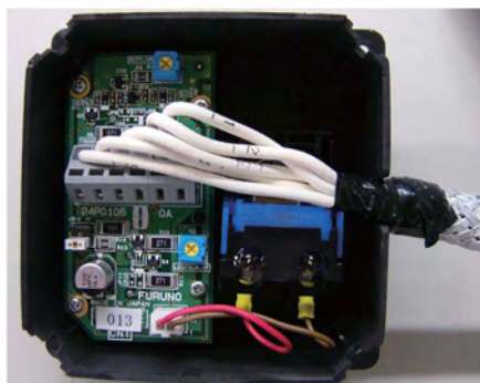
2) Process cable and connect cable to WAGO terminal block. Use terminal opener (inside Processor Unit) to open terminals. (Shown: Timer Reset Panel)
